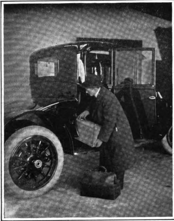
How waste space is utilized in a closed car. The compartment is large enough to house several bags in addition to spare tires, tools, etc.
